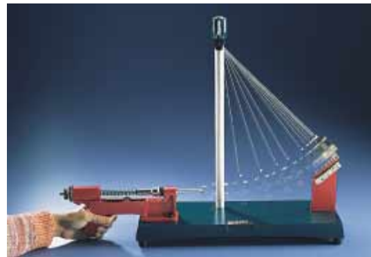
Figure 9.11 (a) Diagram of a ballistic pendulum. Note that \mathbf{v}_{1i} is the velocity of the bullet just before the collision and \mathbf{v}_f = \mathbf{v}_{1f} = \mathbf{v}_{2f} is the velocity of the bullet + block system just after the perfectly inelastic collision. (b) Multiflash photograph of a ballistic pendulum used in the laboratory.
