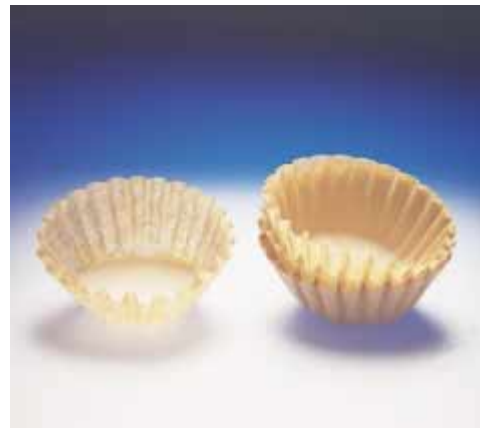
Pleated coffee filters can be nested together so that the force of air resistance can be studied.
