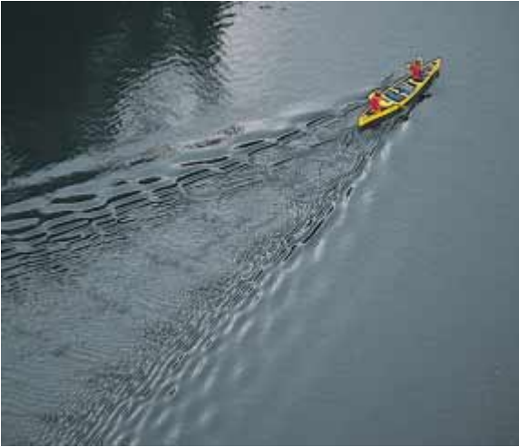
Figure 17.13 The V-shaped bow wave of a boat is formed because the boat speed is greater than the speed of the water waves. A bow wave is analogous to a shock wave formed by an airplane traveling faster than sound.
