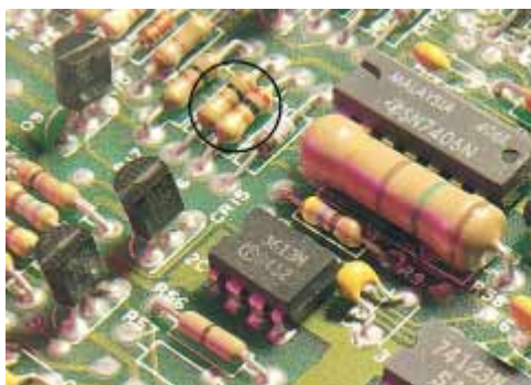
Figure 27.6 The colored bands on a resistor represent a code for determining resistance. The first two colors give the first two digits in the resistance value. The third color represents the power of ten for the multiplier of the resistance value. The last color is the tolerance of the resistance value. As an example, the four colors on the circled resistors are red (= 2), black (= 0), orange (= 10^3 ), and gold (= 5%), and so the resistance value is 20 \times 10^3 \Omega = 20 \text{ k}\Omega with a tolerance value of 5% = 1 \text{ k}\Omega . (The values for the colors are from Table 27.2.)
