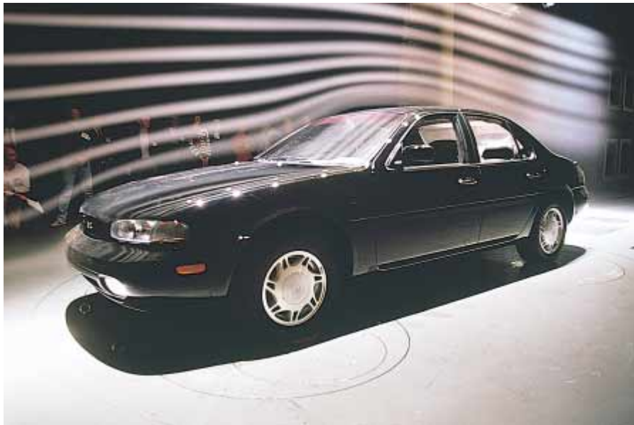
Figure 15.14 Laminar flow around an automobile in a test wind tunnel.
